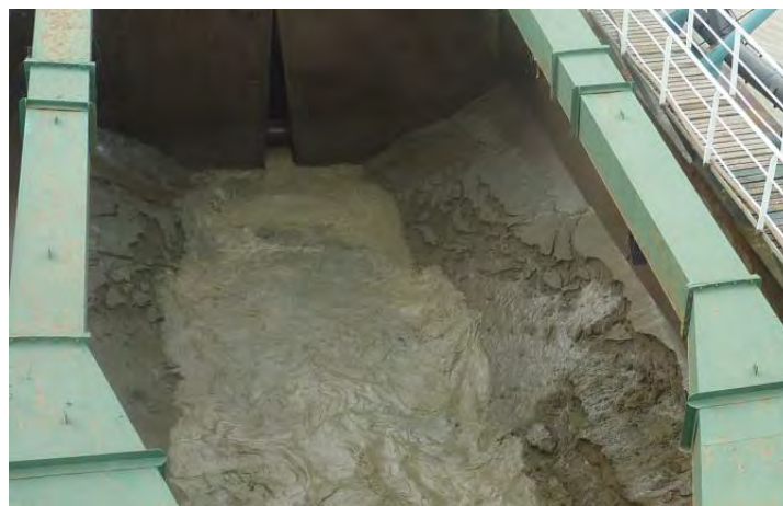
Figure 3.4-6 Mud in Hopper Bottom After Dumping (Pump RPM 1,250R/M)
