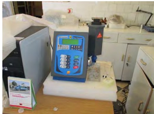
2, BWB flam photometer Na, K, Ca, Mg, Ba,
