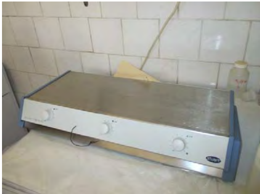
9, SBH200 block heater COD reactor
