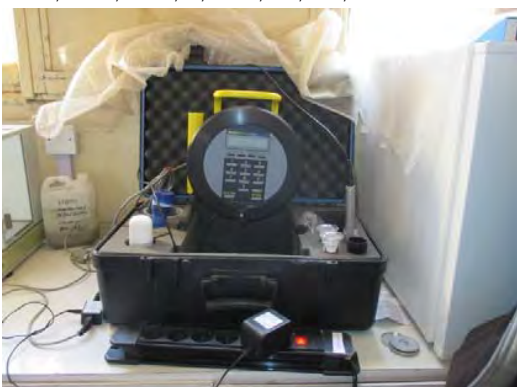
3, Portable PHA-100plus Hydrocarbon
