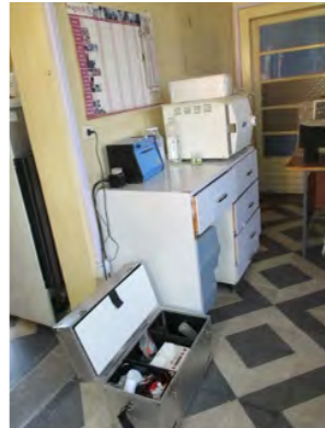
10, Bacteriological incubators for faecal and total c. bac Coliform bacteria
