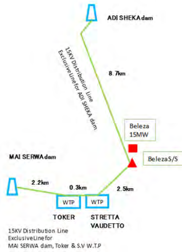
Figure-3: Exclusive distribution lines required in the future plan
