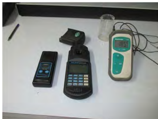
Toker W.T.P pH and turbidity and residual chlorine equipment There is no reagent of residual chlorine equipment.
