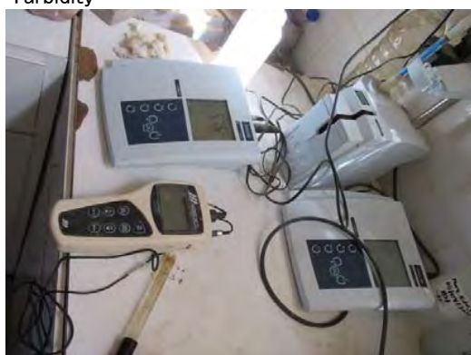
6, Digital EC/TDS/PH meter EC, TDS, PH,
