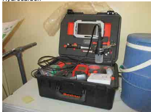
5, Portable HM3000 metalzer Heavy metals (Not trained person)
