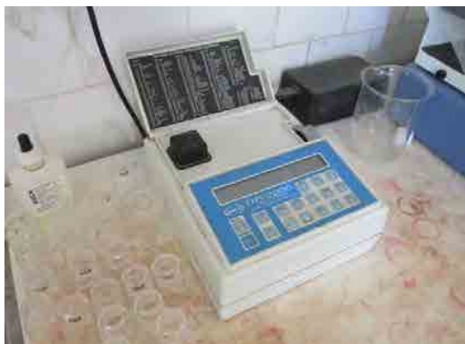
1、Dr/2000 and Dr/2800 spectrophotometer NO3, NO2, SO4, F, NH3, Fe, Mn, Free Cl2
