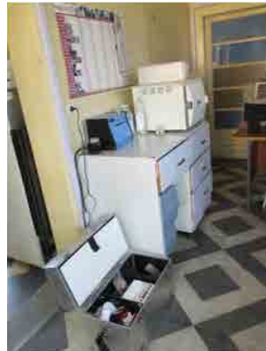
10, Bacteriological incubators for faecal and total c. bac Coliform bacteria
