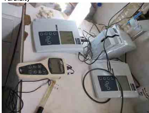
6, Digital EC/TDS/PH meter EC, TDS, PH,
