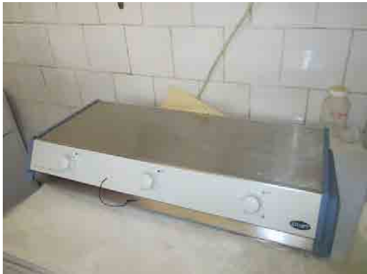
9, SBH200 block heater COD reactor
