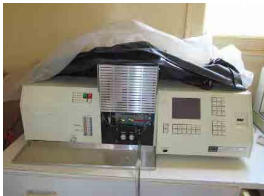
7, 210/211 VGP atomic absorption spectrophotometer Heavy metals (Not trained person)
