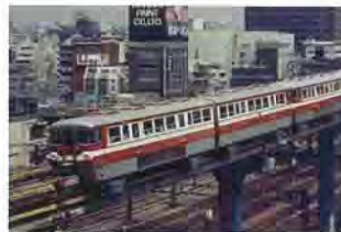
■ 500 Series (1969~1991) First monorail to adopt tandem design bogies (26 cars produced)
