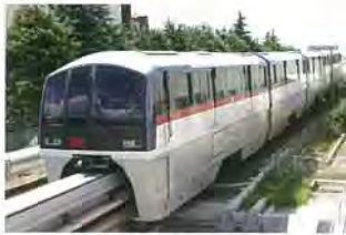
■ 2000 Series (1997~) First monorail to adopt VVVF inverter (24 energy-saving cars produced)
