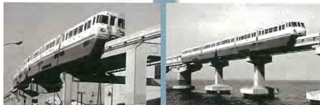
■ 500 Series (1969~1991) First monorail to adopt tandem design bogies (26 cars produced)
