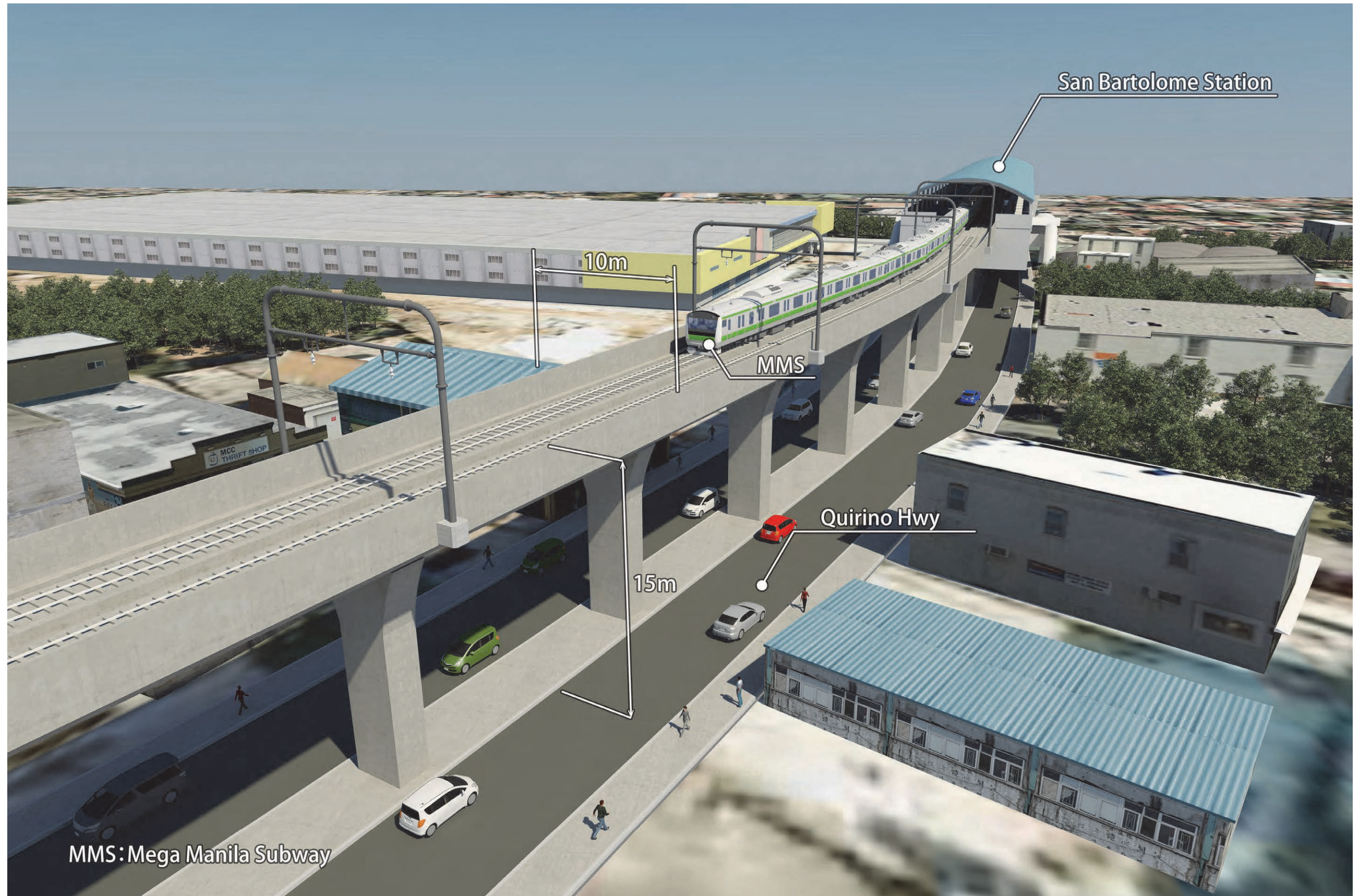
Figure Annex-B (7) Typical Elevated Section along Existing Road (Quirino Highway – Option A in North Zone)
