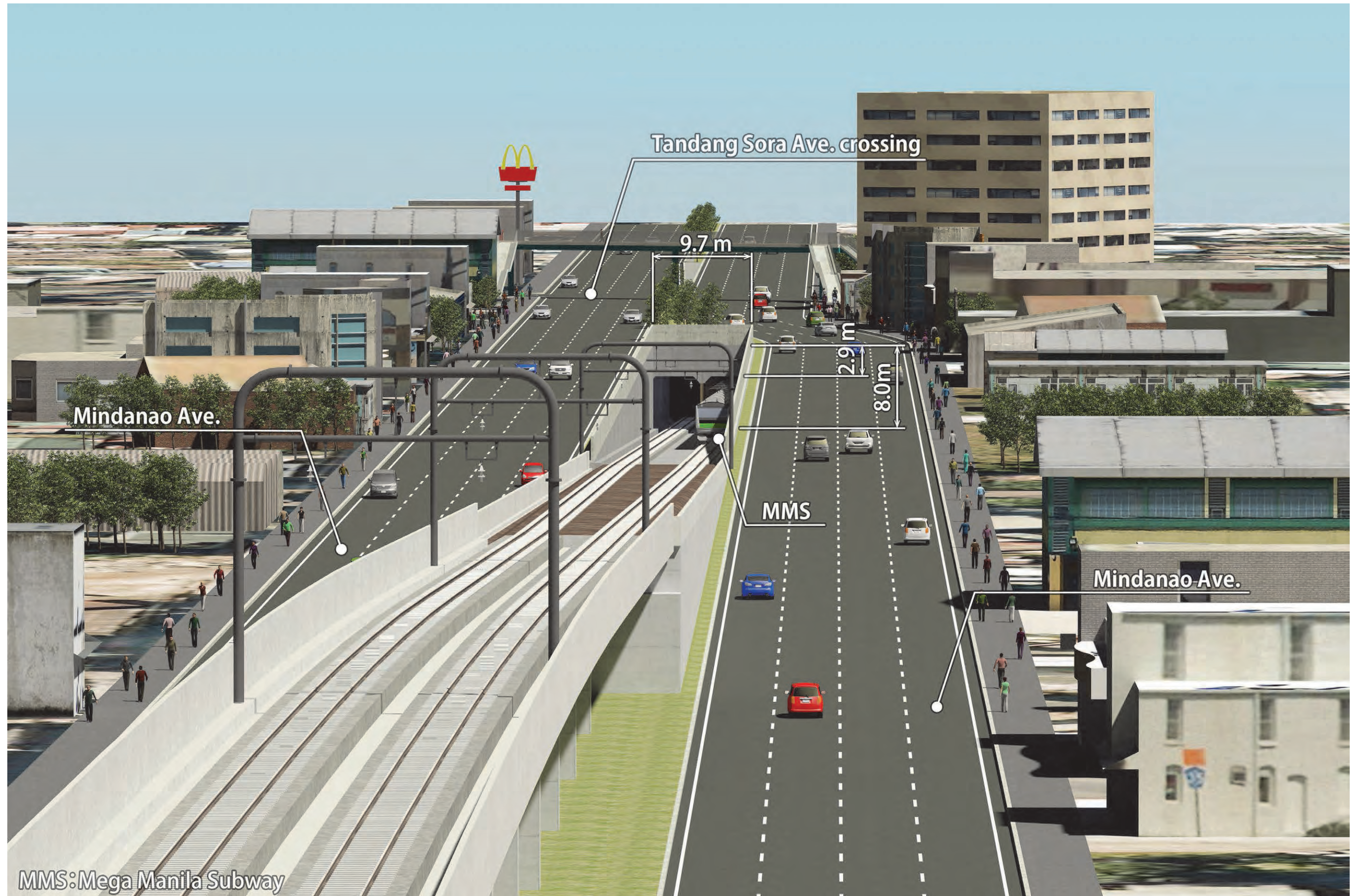
Figure Annex-B (6) Transition Section from Underground Structure to Elevated Structure (Along Mindanao Avenue – North Part of Central Zone)
