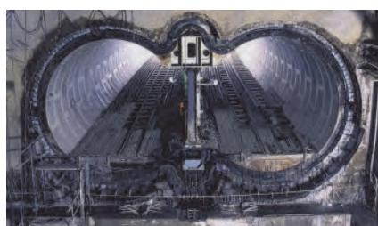
H&V (Horizontal Variation & Vertical Variation) Shield Machine with 4-circles
