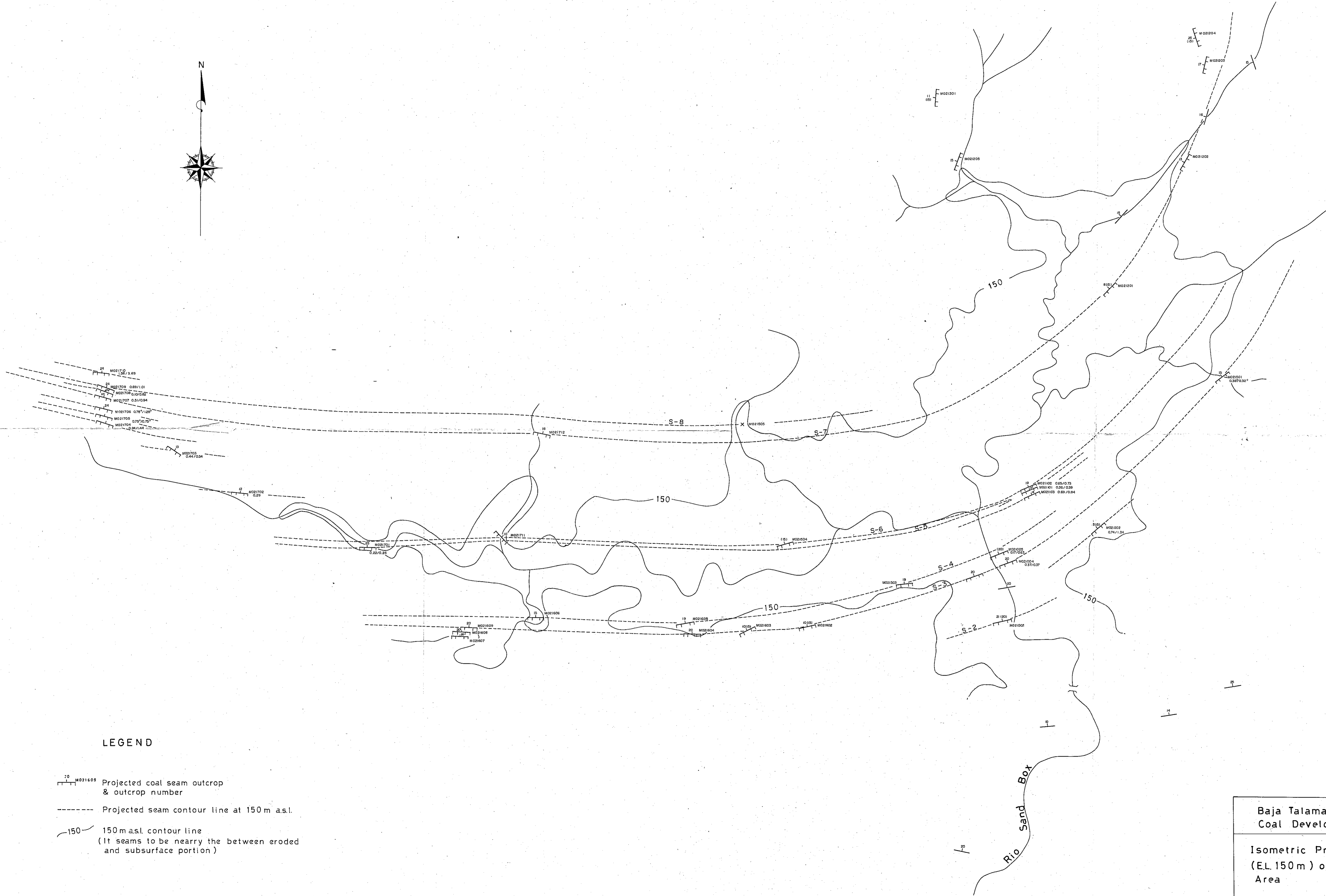
Figure 8 Isometric Projection Map at 150 m a.s.l. of Main coal Seams in Sand Box Area
