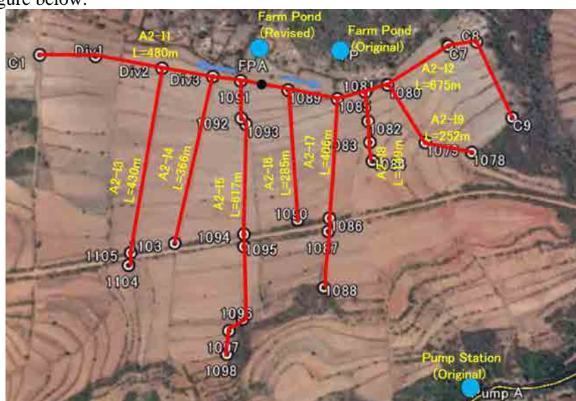
Figure Existing Irrigation Canal in Block A
