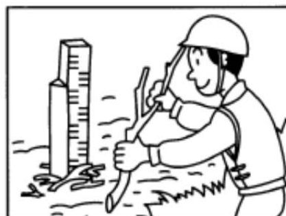
Remove objects/debris from staff gauge Figure 2-11 Cleaning Staff Gauges by an Observer
