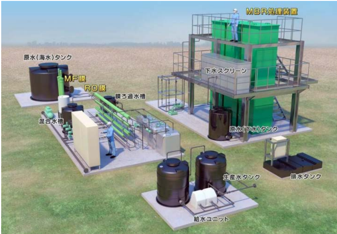
Fig. 3 Image of plant layout of Membrane Bioreactor + Reverse Osmosis Membrane
