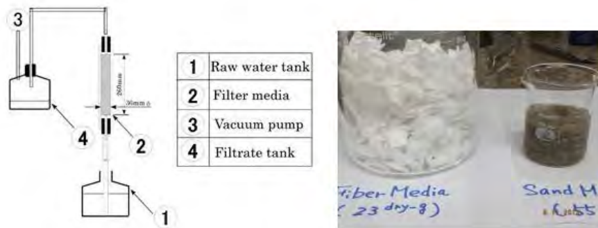
Figure 5.2-6 Experimental Apparatus and Filtering Media
