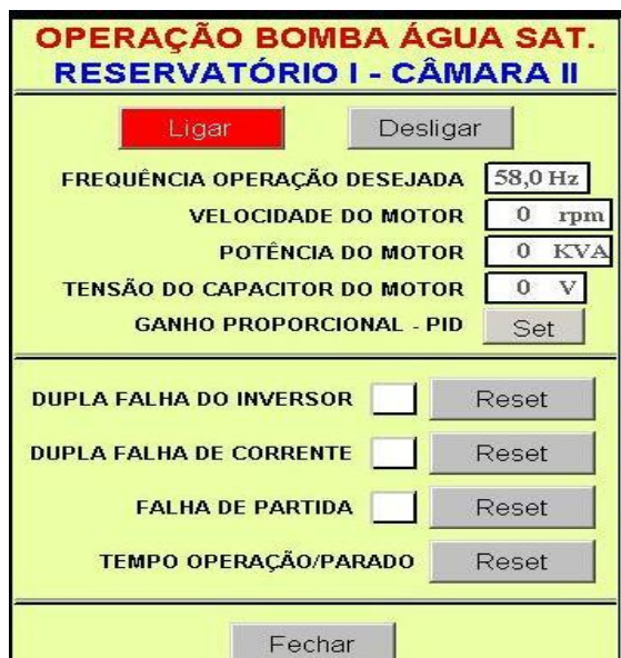
COMMAND PANEL OF THE SATURATED WATER PUMP
