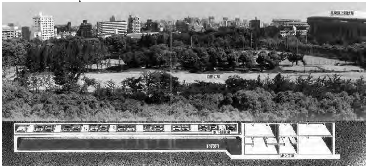
Figure 7.2. Example of an Underground Water Distribution Plant
