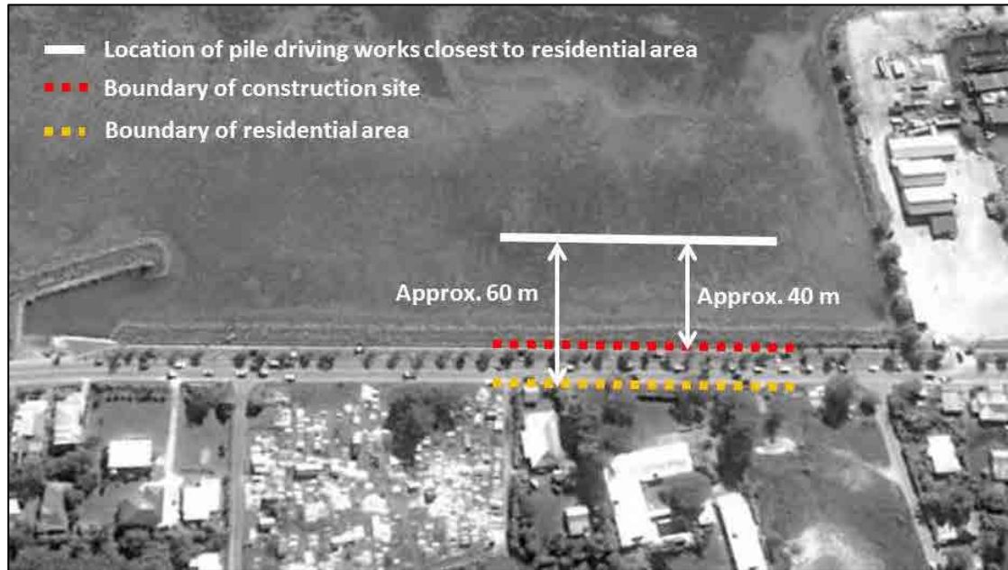
Figure 6-1 Distance between pile-driving works and the boundary of construction site and residential area (under worst-case scenario)
