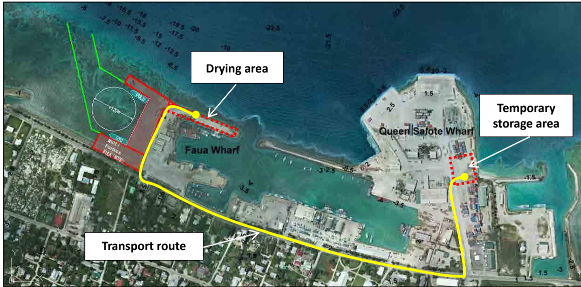
Figure 3-5 Handling process of the excessive dredged material
