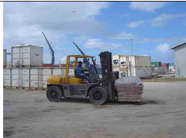
Photo 1-8: Forklift (8 tons weight) for cargo handling
