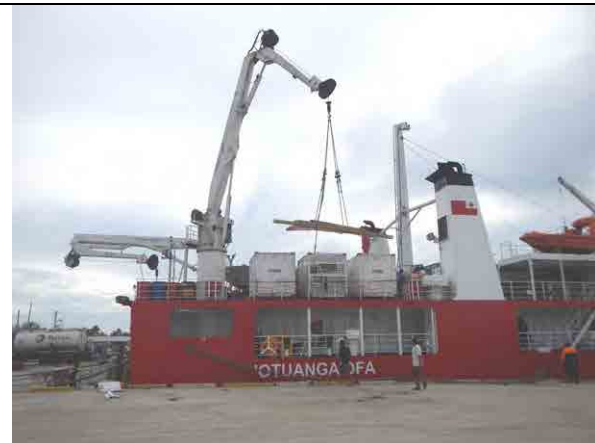
Photo 1-9: Cargo Loading by Ship Crane MV Otuanga'ofa has two ship cranes.
