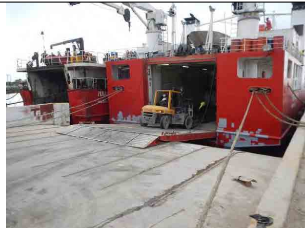
Photo 1-7: Cargo Loading into MV Otuanga'ofa Containers and bulk cargoes are loading by forklift.
