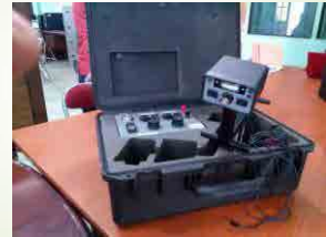
D 305 PVC pipe locator
