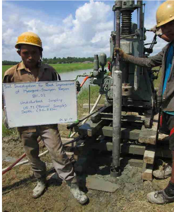
Piston Undisturbed Sampling
