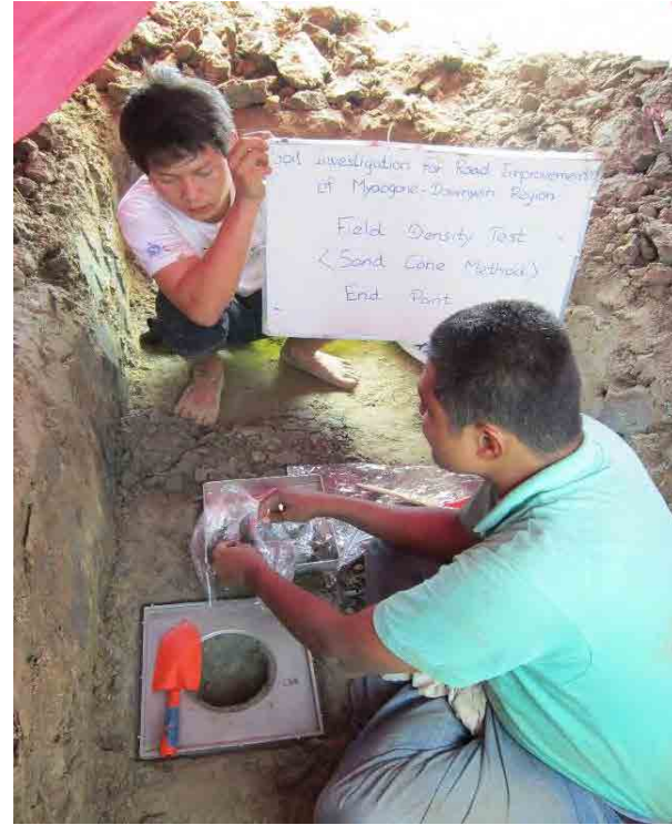
Preparation for Field Density Test
