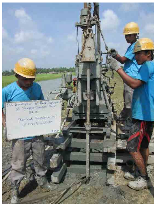
Photo - 3.2 : View of Standard Penetration Test and SPT Sample
