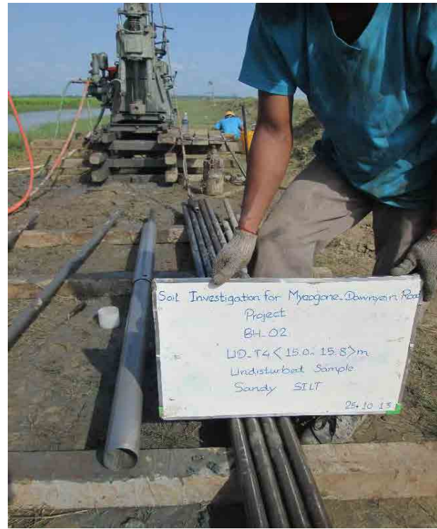
Piston Undisturbed Sample
