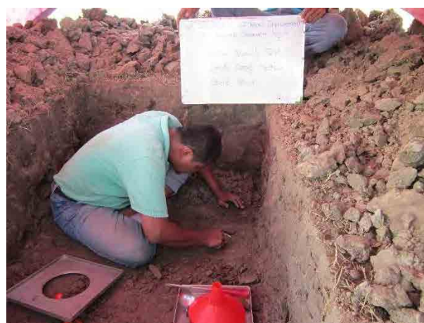
Photo - 3.3 : View of Carrying out Filed Density Test
