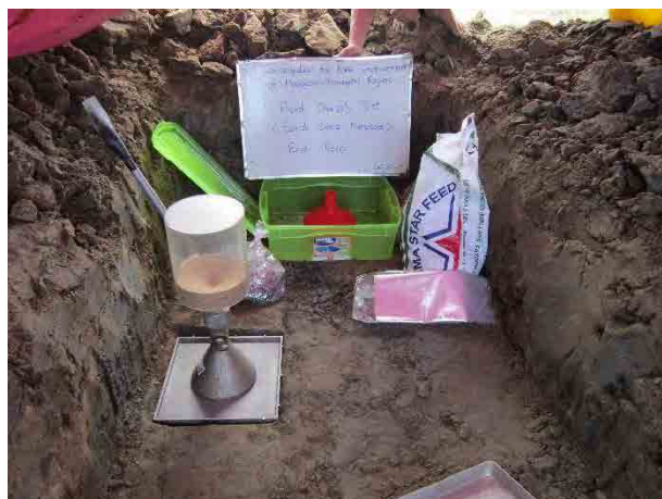
Photo - 3.3 : View of Carrying out Filed Density Test
