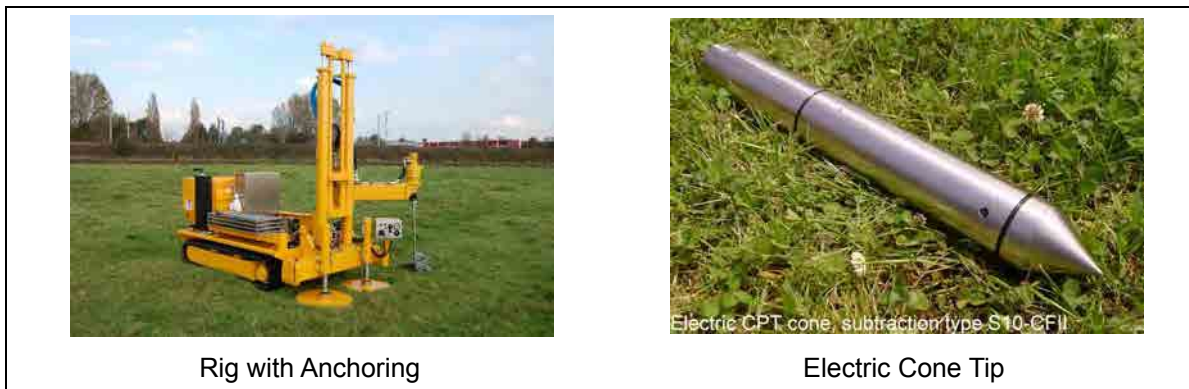
Figure 2-4 Examples of electric cone penetrometer apparatus 9)
