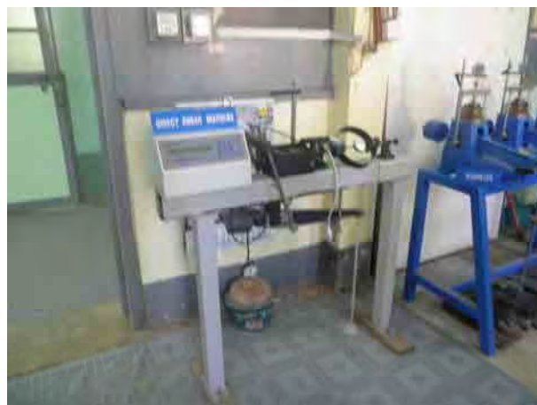
Figure 2-28 Direct shear apparatus in soil research laboratory, Public Works
