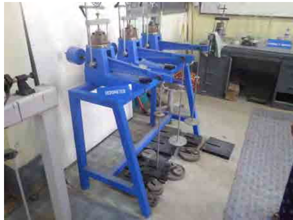
Figure 2-30 Oedometers in Bridge Research Laboratory, Highway Department, MOC
