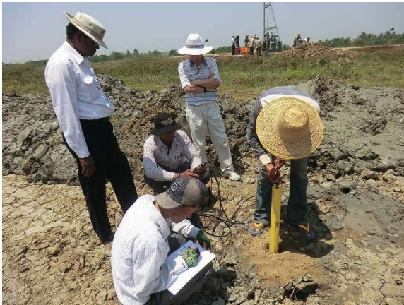
Practical Training of Inclinerometer
