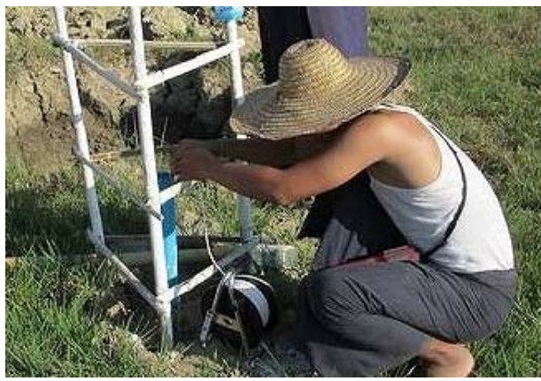
Measuring of Underground water level by electric detector
