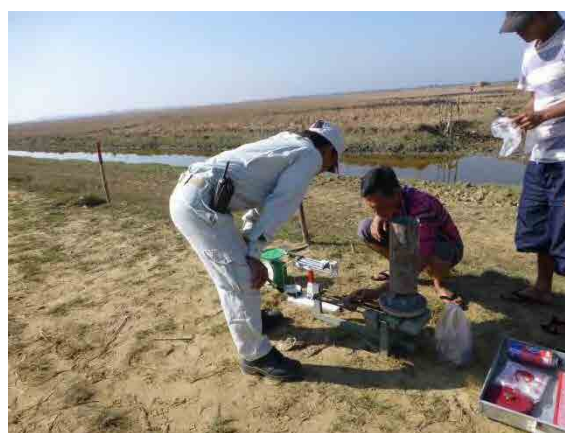
Photo-.22 Dry Density Test of Existing Subgrade in situ
