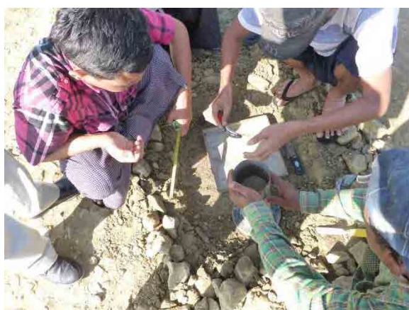
Photo-.22 Dry Density Test of Existing Subgrade in situ
