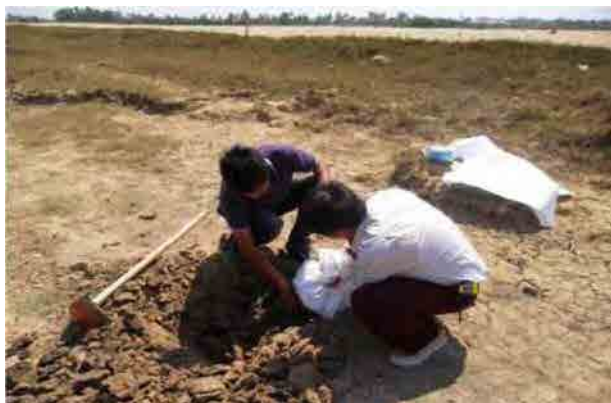
Photo-2.1 Taking sample soil for laboratory test
