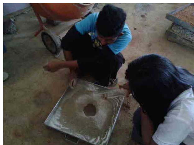
Photo-3.2 Mixing Test of Stabilized Materials for Subbase
