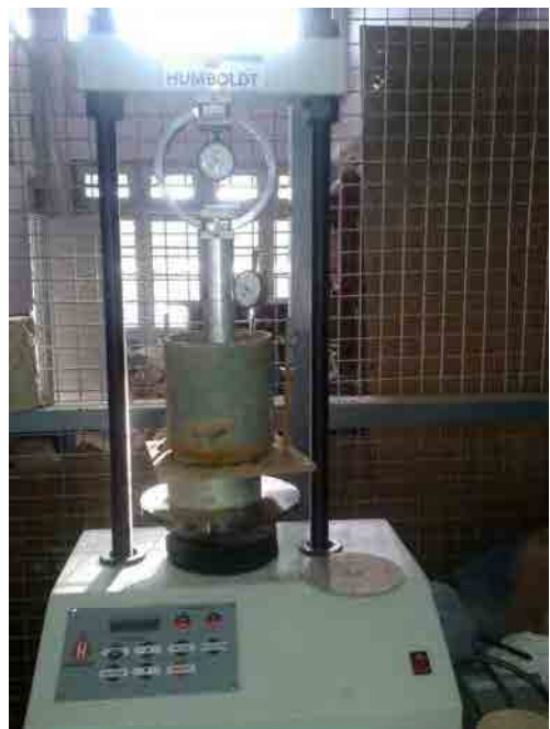
Photo-3.1 CBR Test On Stabilized Subgrade Material
