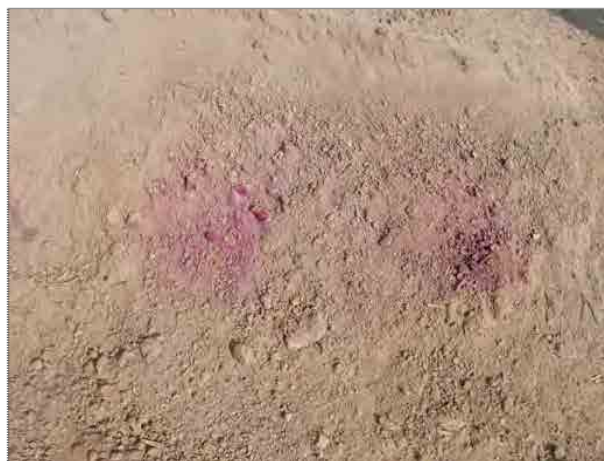
Figure 4.2.5 Turned Color of the Material due to Acid-Base Reaction
