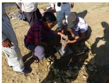
Degree of confirmation test (Sand replacement method)
