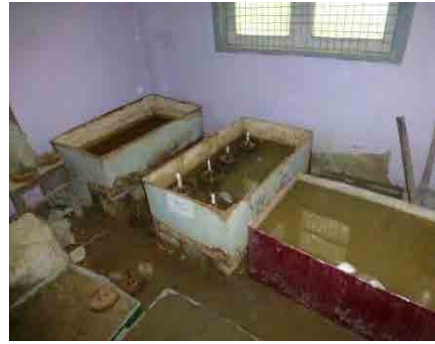
Curing of Test Pieces for CBR test
