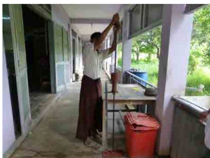
Checking of Cone type penetration tester
