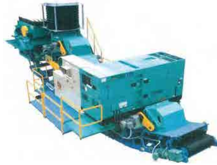
Photo 10 Soil Mixing Plant (Fixed Type)
