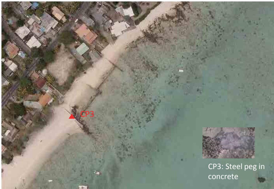
Control Station CP3 on Groyne
