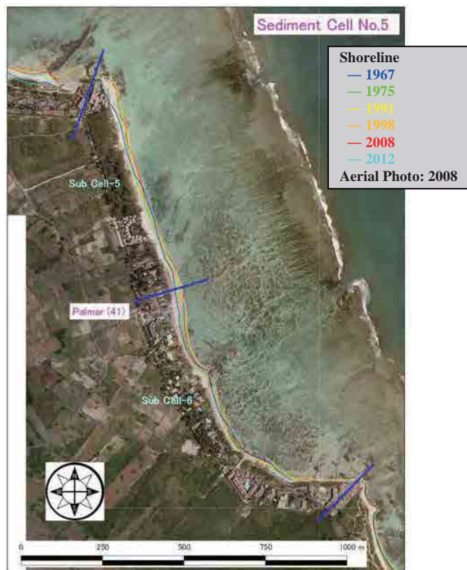
Source: This figure was processed by JICA Study Team based on Satellite image obtained from MHL. Figure 1.10 Area of analysis (Sediment Cell No.5, Sub Cell-5-6)
