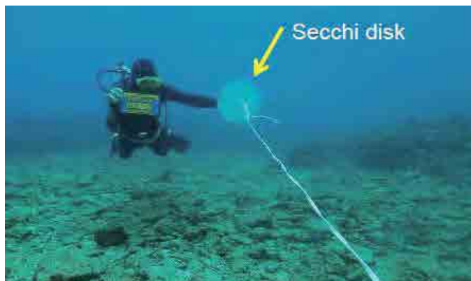
Figure 4.3.1 Measurement of Transparency by Secchi Disk in Lagoon
