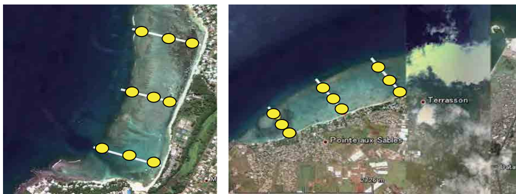
Figure 4.2.1 Typical Arrangement of Water Quality Monitoring Points in a Lagoon
