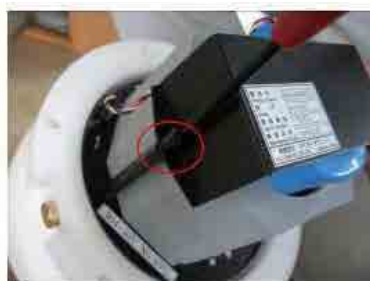
Photo.8 Taking off a settle board.
