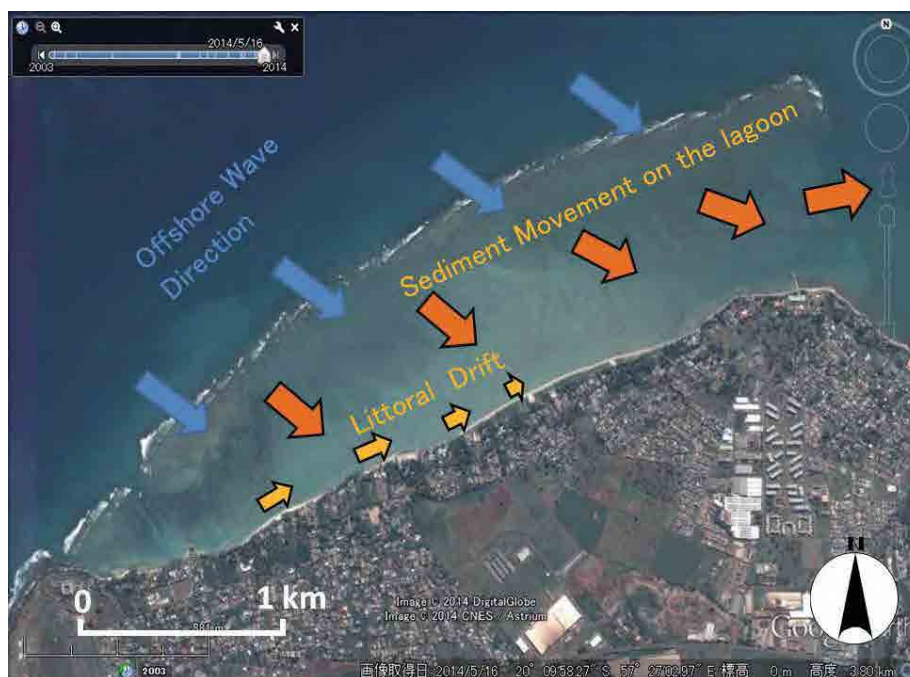
Figure 12.3.1 Wave and Littoral Drift Pattern at Pte. aux Sables
