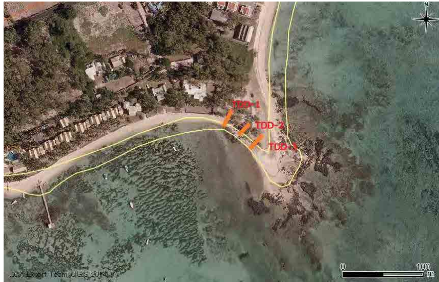
Figure 5.3.5 Arrangement of Transect for Beach Monitoring
