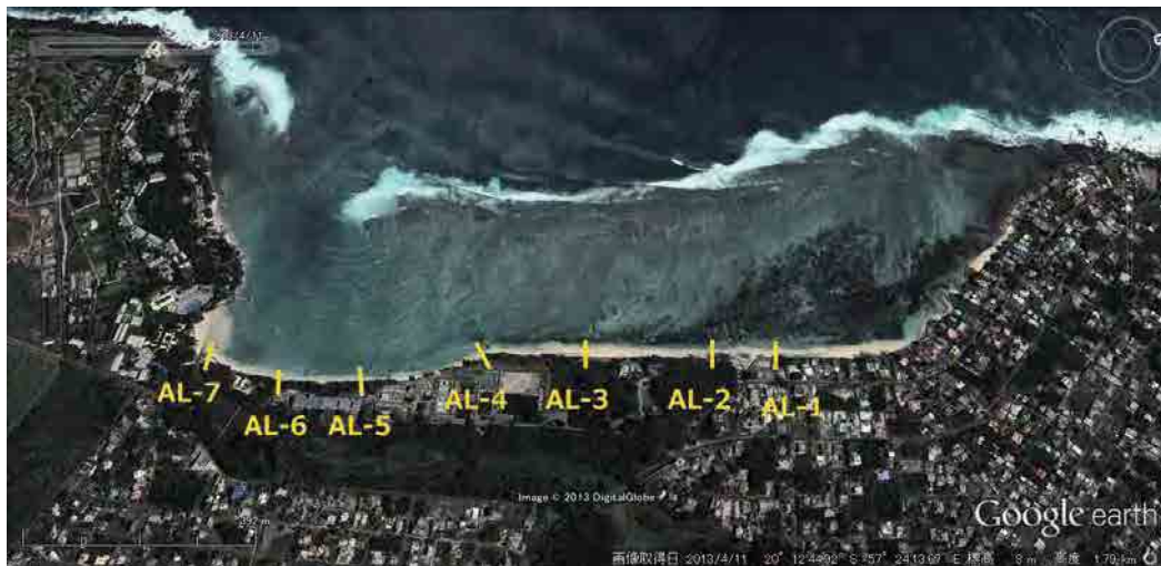
Figure 11.3.4 Arrangement of Transect for Beach Monitoring
