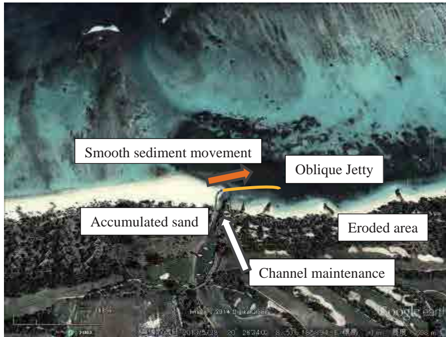
Figure 9.4.1 Channel Maintenance Plan at Le Morne
