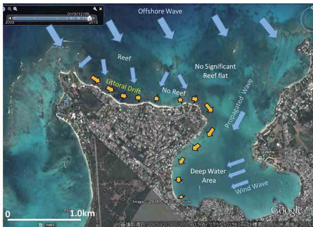
Figure 2.3.1 Waves and Littoral Drift Patterns at Pte. aux Cannoniers
