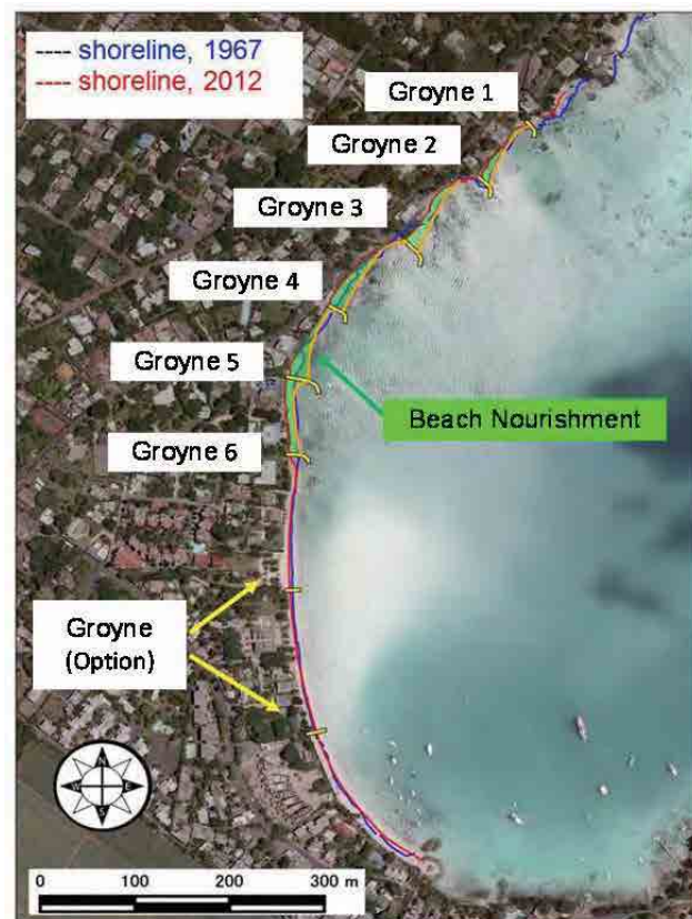
Figure 2.4.3 Short Term Measures at East Eroded Area
