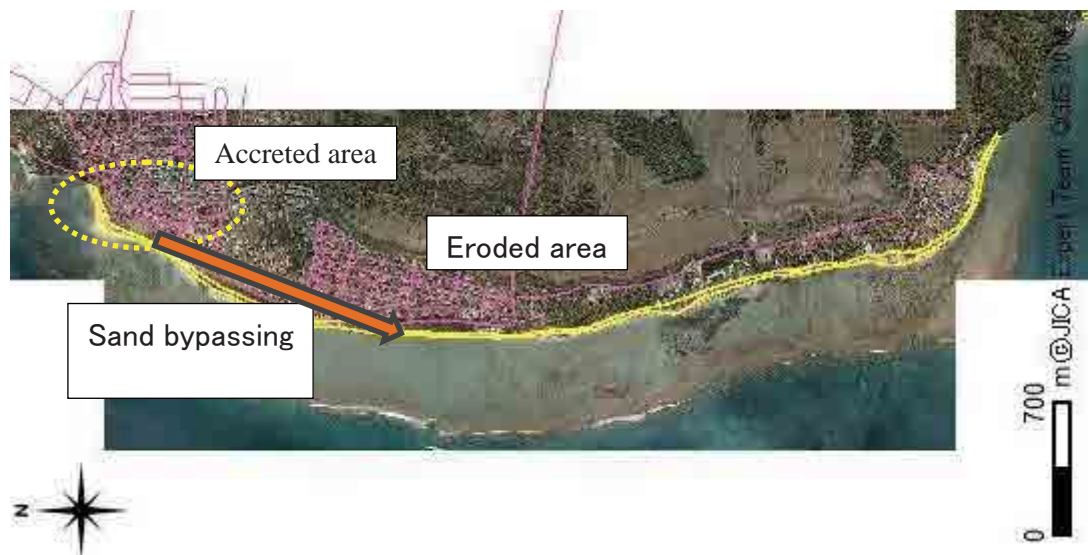
Figure 10.4.1 Arrangement of Measures at Flic en Flac
