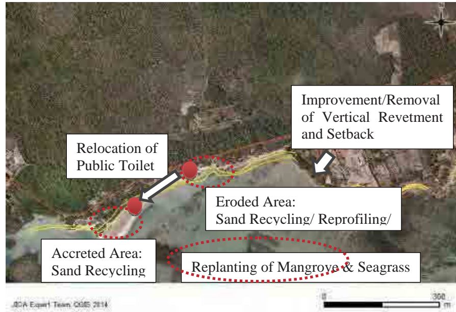
Figure 4.4.1 Arrangement of Measures at Bras d'Eau
