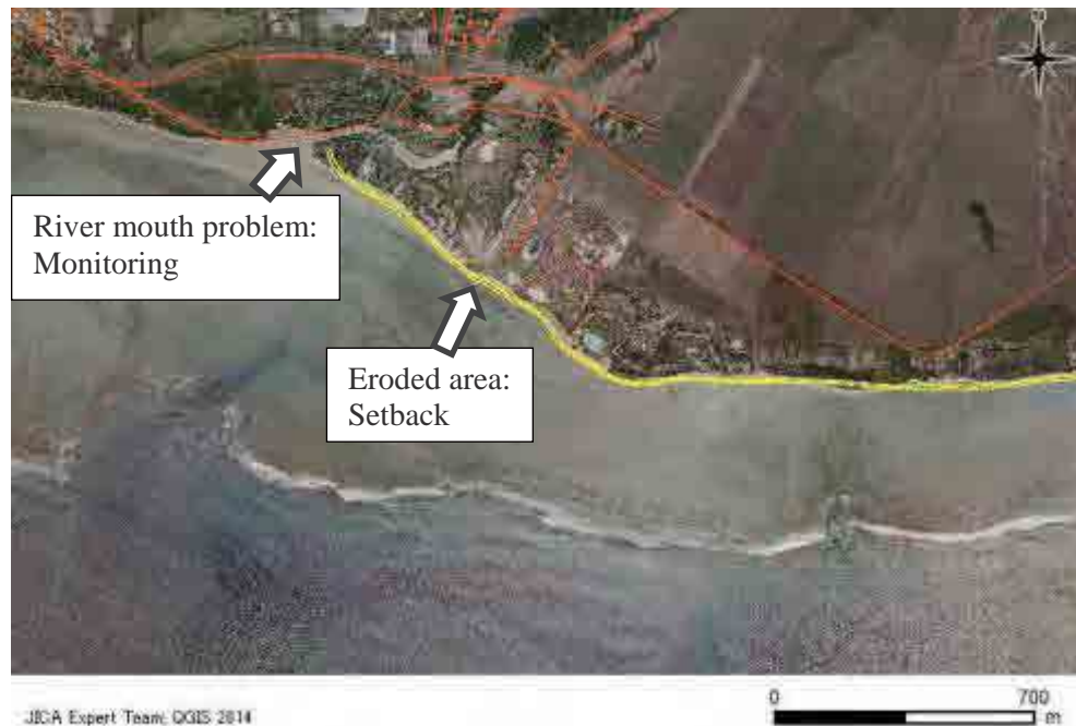
Figure 8.4.1 Arrangement of Measures at Bel Ombre
