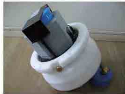
Photo.4 Put sponge under the electromagnetic current speed meter
