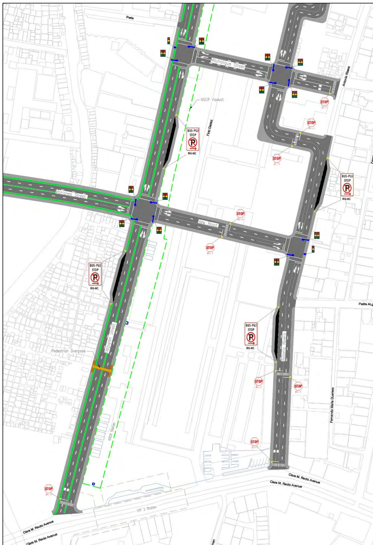
Figure 3.10.20 Improvement of Pedestrian Crossings, Signs, and Pavement Markings (South side of Tutuban PNR Property)
