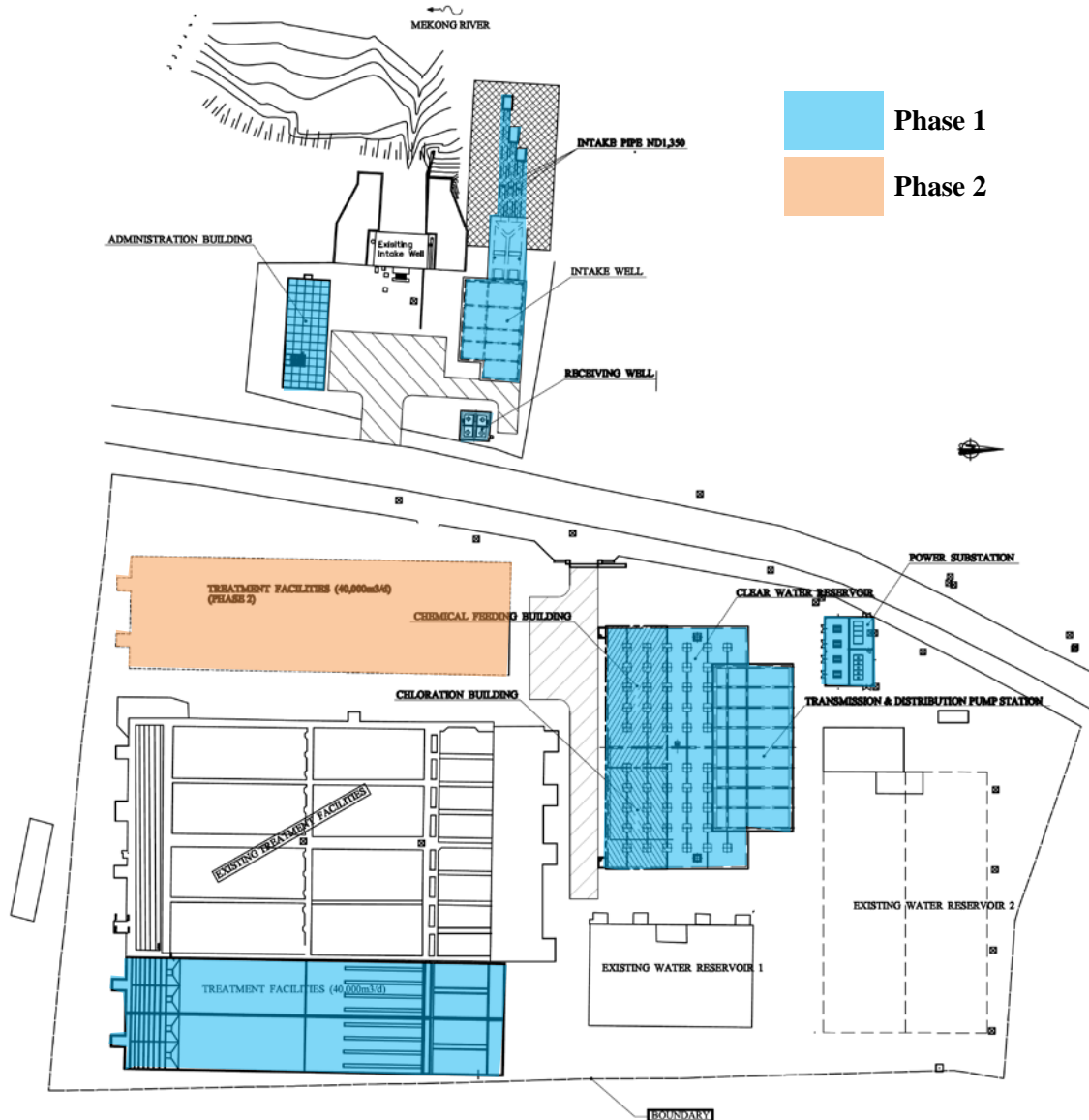
Figure 5.1 Layout Plan of the Expanded Chinaimo WTP and Raw Water Intake Pump Station
