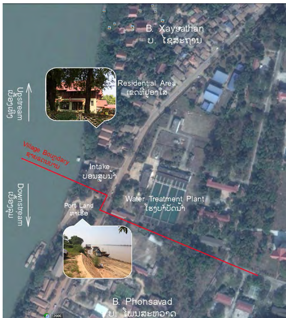
Figure 6.6.1 Location of New Intake in the Existing Chinaimo Water Intake
