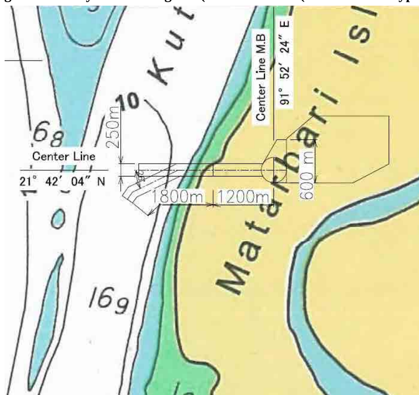
Figure 4.4-2 Layout Planning A-2 (Matarbari Site (Excavated Type))
