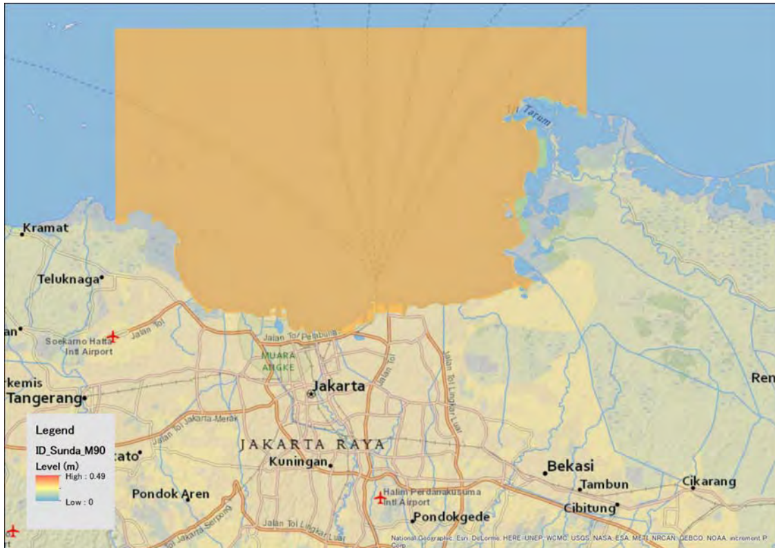
Figure 3.7 Distribution of Tsunami Simulation result for Mw 9.0 earthquake in and around Jakarta, Indonesia
