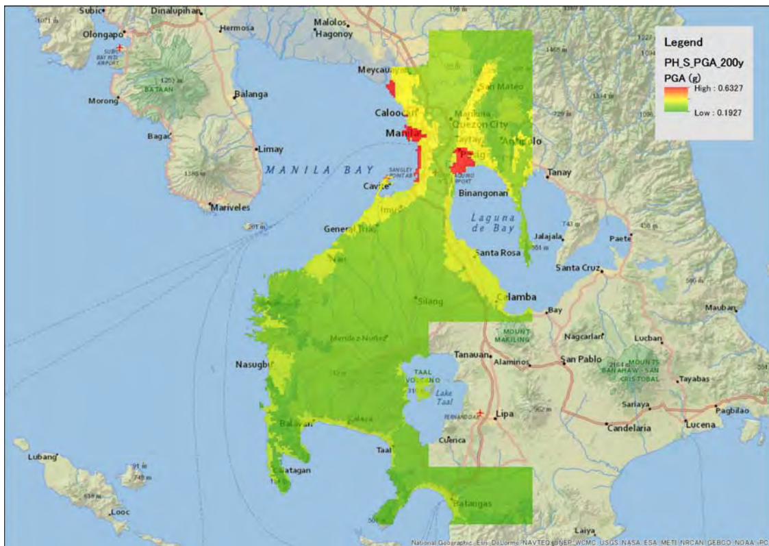
Figure 3.2 Ground Shaking Simulation for 200 years return period in and around Manila, the Philippines
