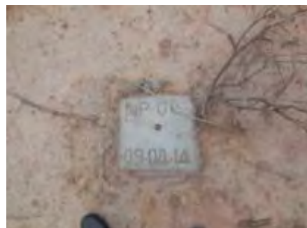
Benchmark Set at Ongoing Railway Extension Construction Site at Northern End
