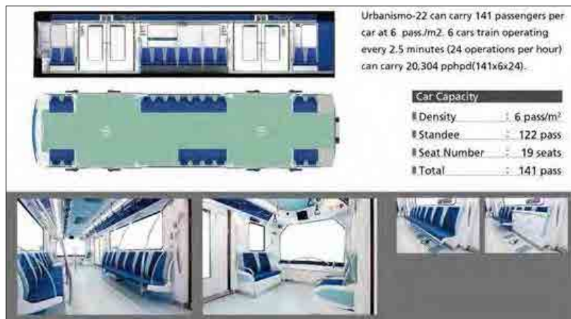
Figure 11.3.2 Internal Layout of the AGT Railcars
