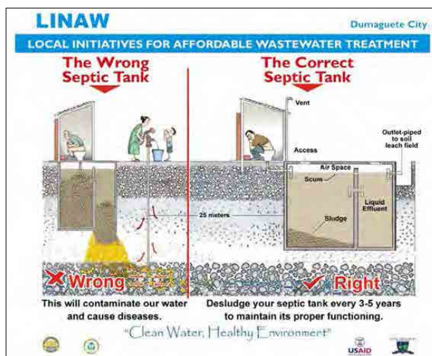
Figure 6.4.2 Wrong and Correct Designs of Septic Tank
