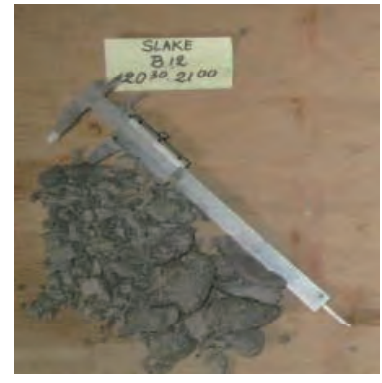
Fragment Type Retained : Type II :Retained materials consist of large and small pieces
