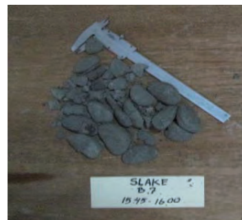
Fragment Type Retained : Type II :Retained materials consist of large and small pieces
