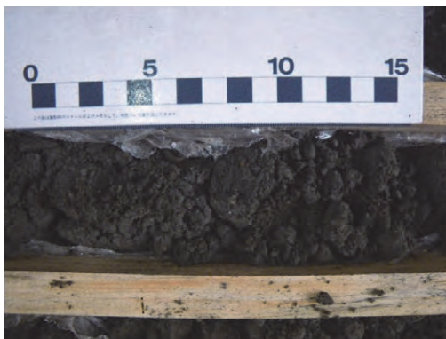
Photo-2.12 Boring core of Fan Deposit
