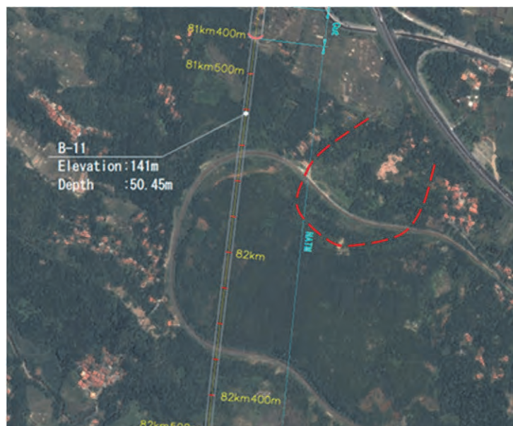
Figure 7.2-4 Existing Landslide Area Sta. 81 km
