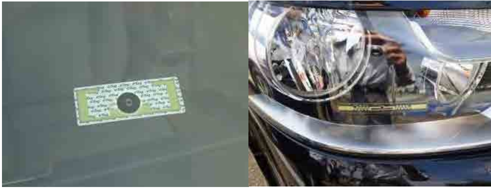
Figure.2.100 RFID Tag Installed inside Windshield and on Headlight
