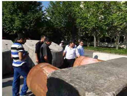
Observation of damaged members stored by Public Works Research Institute
