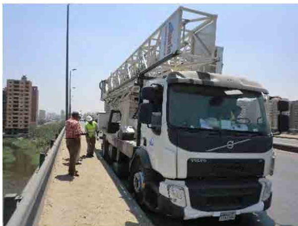
Picture 1-2 Bridge Inspection Vehicle
