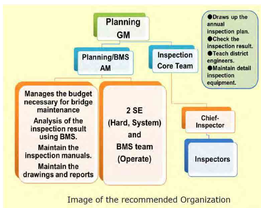
Figure 2-4 Proposed bridge maintenance management organization
