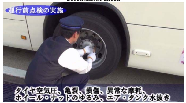
Tire and loosening nuts check
