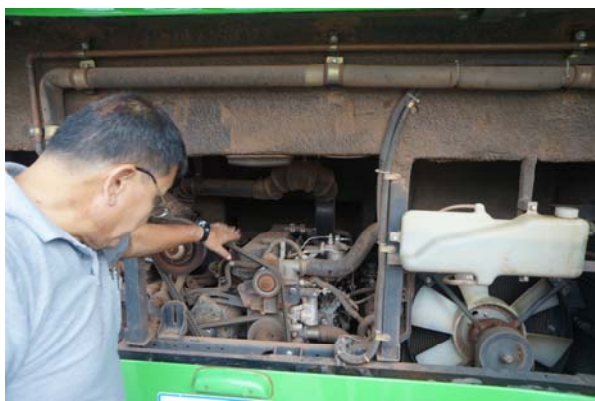
Check Engine Belt by hand
