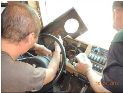
Installation of Digital Tachograph (24 - 29 October, 2012)
