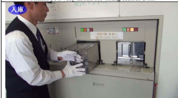
Driver does not touch any cash but automatic cash collection system handle cash.
