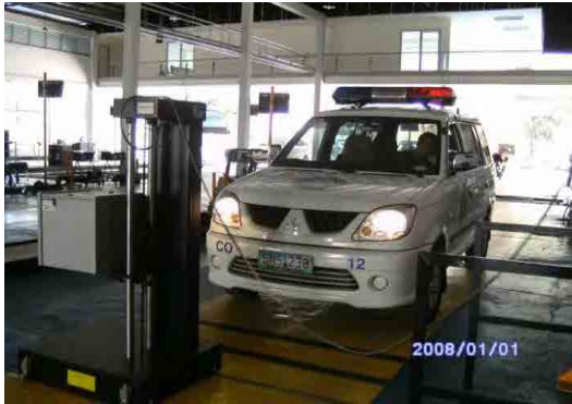
Figure2-25 Headlight test Equipment
