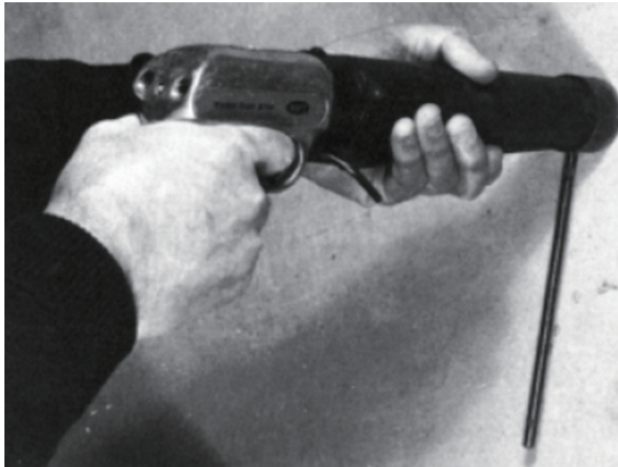
Rebound Hammer Test
