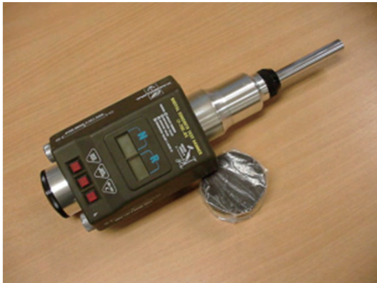
Rebound Hammer Test
