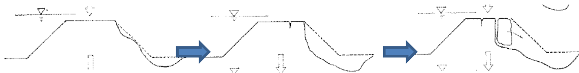
Figure 7.5-6 Failure Progress of Grass sodding Dike
