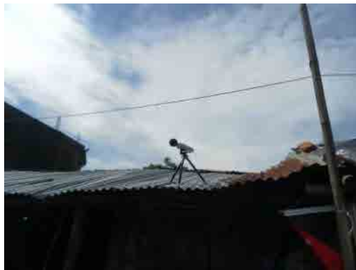
Figure: Noise Sampling at Ilisha Bazar (Between Eidmoni and Badarkhali)
