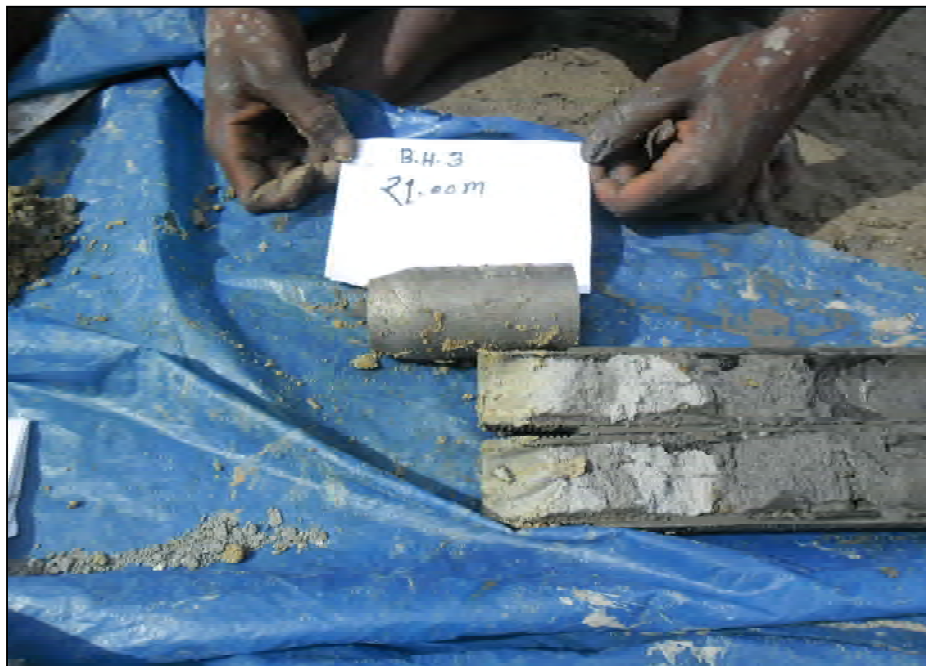
Figure -2 Soil Sample collection at Matarbari
