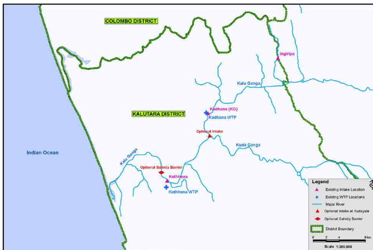
Figure 4.4.1: Kalu and Kuda Rivers, Existing and Alternative Locations of Intakes and Planned Salinity Barrier
