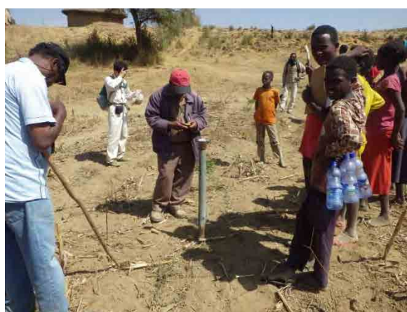
Thermal Gradient Well (TG Well) found at the foot of Finkilo site
