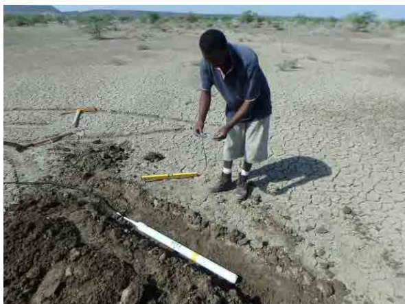
Setting of Induction Coil for MT Survey
