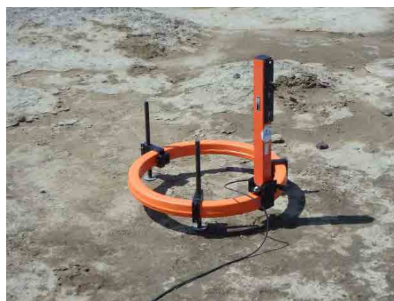
Setting of Inductor Coil for TEM Survey
