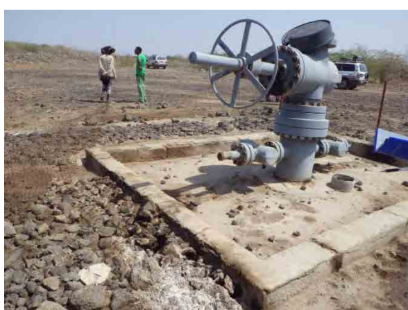
Well head of TD-6; BOP is tilting.
