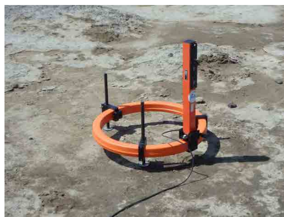
Setting of Inductor Coil for TEM Survey
