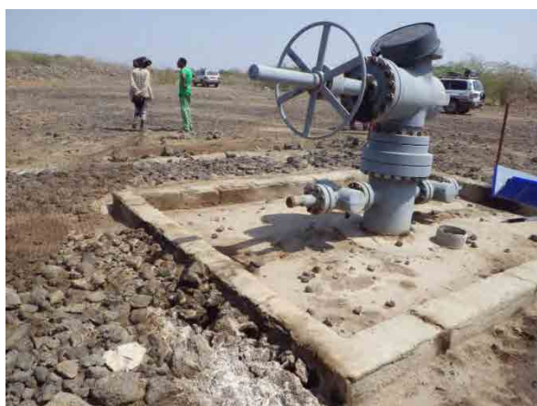
Well head of TD-6; BOP is tilting.
