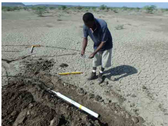
Setting of Induction Coil for MT Survey
