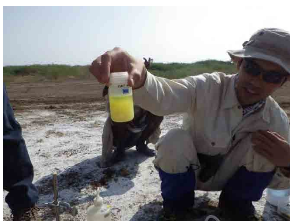
The color of sample shows Containing of Sulfur in collected gas
